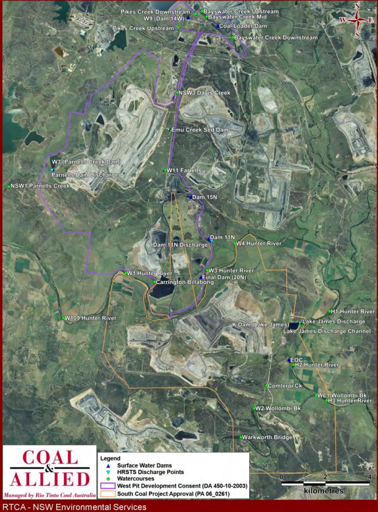
Figure 22: Surface Water Monitoring Location Plan
